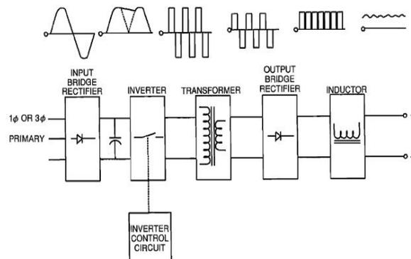
**Figure.1 block diagram of inverter welding machine**
