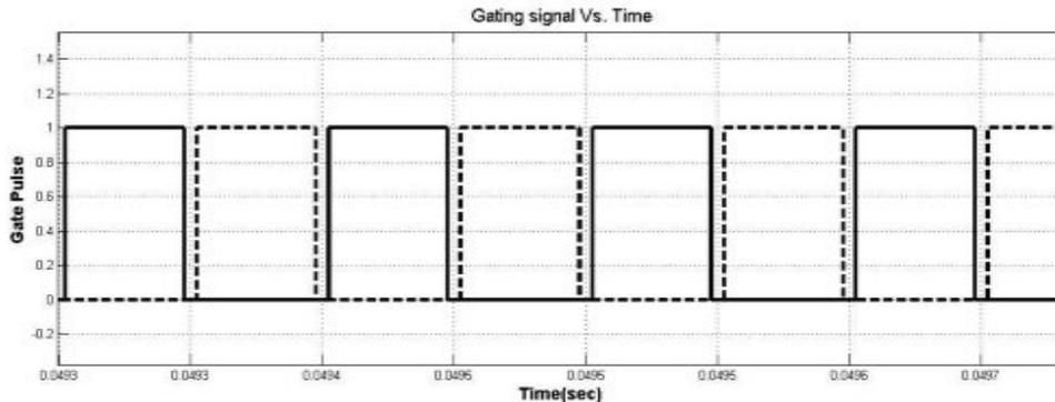
Figure.3.2 gate pulse of H-bridge inverter
