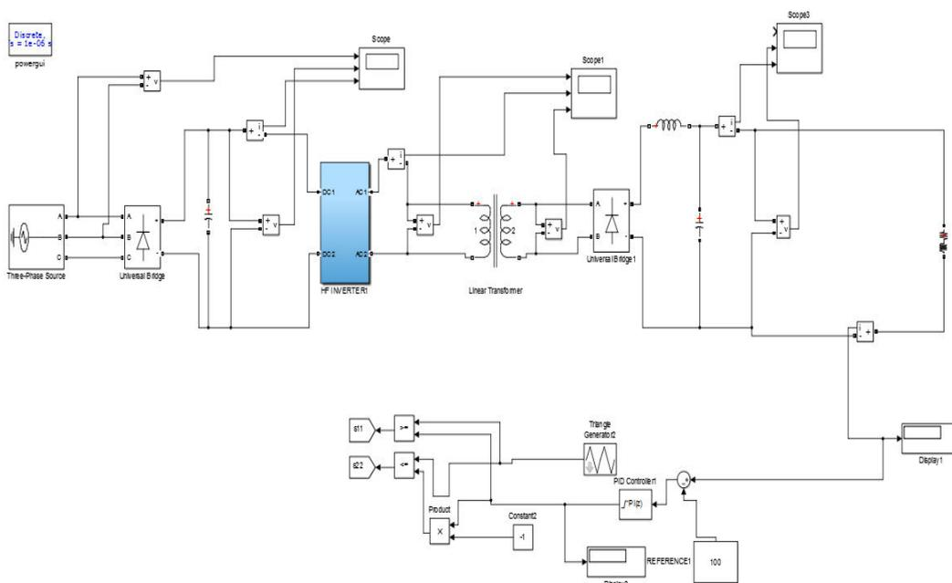
Figure.3 simulationwelding circuit in constant current mode of 3-phase, 60volt, 100 ampere
