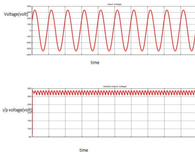
Figure.3.1 waveforms of ouput voltage for 3-phase rectified voltage
