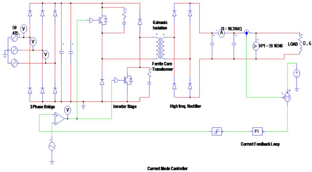
Figure.4 simulation circuit of welding circuit with PSIM SOFTWARE.
