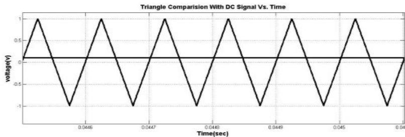
Figure.3.1 triangular comparison with dc signal
